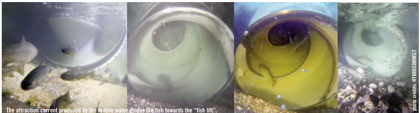
The attraction current produced by the motive water guides the fish towards the "fish lift".
